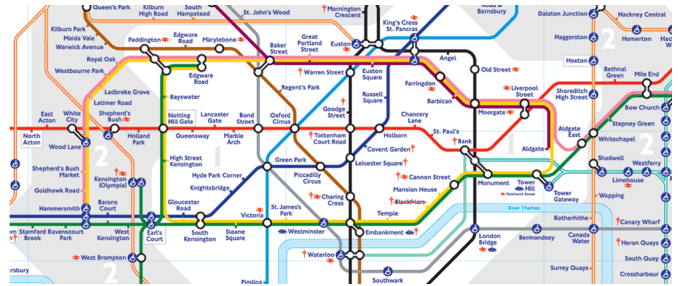
Fig. 1. An example of the classic octilinear schematic representation used in most metro maps today and originally developed for the London Underground map by Harry Beck in 1931.
