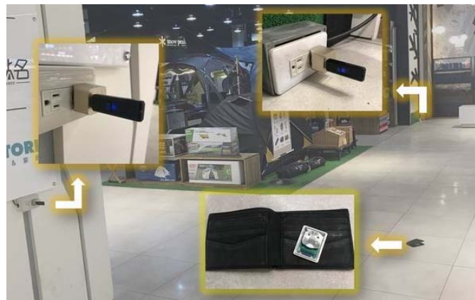
Fig. 5. Installation of static and mobile iBeacon nodes.
